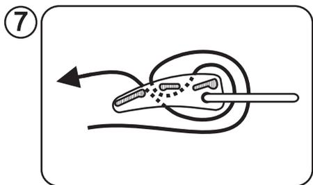
7 Cross section view of how the cam band should be threaded through the cam buckle.
