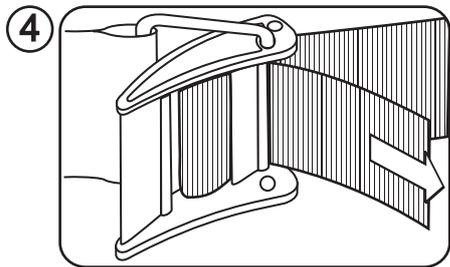
4 The belt can now be tightened against the cylinder by pulling on the webbing.
