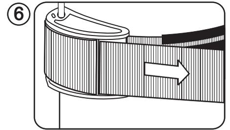
6 To finally clamp the cam buckle, pull on the webbing to make the buckle snap over.
