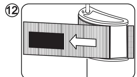
12 To release the cam, just pull on the webbing. The belt can be slid off and on the cylinder without re-adjustment.
