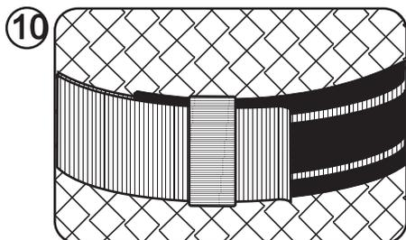
10 If mesh is used on the cylinder, part it to allow the cam band to grip on the cylinder paint surface.
