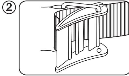
2 Before threading the buckle turn it back against the metal loop. To re-thread the buckle start by pulling the webbing through the metal hoop.
