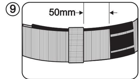
9 Once secure, the webbing is then velcroed down and tucked under the webbing loop, leaving 50mm (2") spare.
