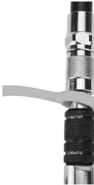
Locking strap fitted incorrectly : below the knurled chrome area
