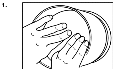
Ensure the filter scrim is clean and undamaged. Push in into the cartridge as far as it will go.
