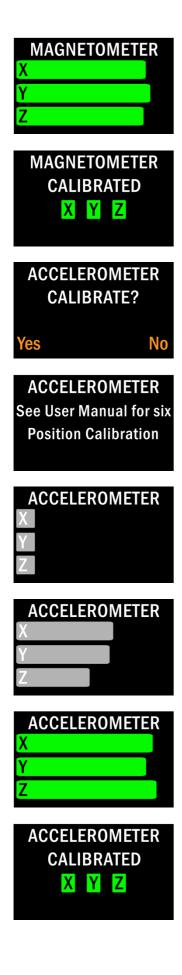
Keep rotating for the full 15 seconds with the goal of achieving a green bar for each plane, indicating that the magnetometer has been subjected to sufficient rotations. The longer the bar, the more accurate the calibration will be.
