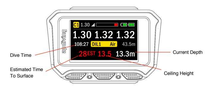
The estimated time to surface and ceiling depth are shown in red, highlighting the fact that the decompression is now estimated due to the ceiling violation.
