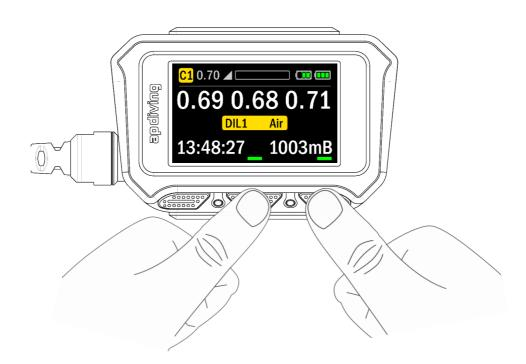
The Power Control screen may be entered at any time, from any screen by pressing the centre and right buttons simultaneously.
