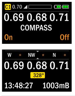
In Surface or Dive Mode, the compass can be accessed by holding the right button for 2 seconds, then press the left button.
