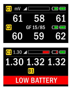
The oxygen sensor mV readings and gradient factor details can be seen by keeping the left button held for a further 2 seconds.
