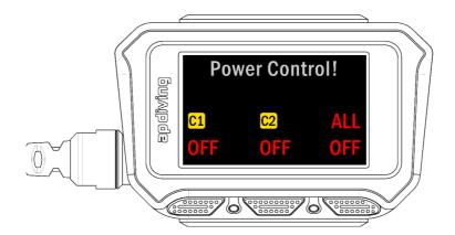
Whilst underwater you cannot turn off the entire system, the ALL OFF option shown at the surface becomes NONE OFF. If one controller is switched off it may be switched on again using the same power control screen.
