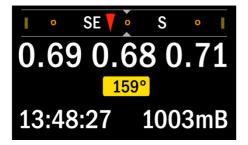
The second example shows a current direction just off the reciprocal heading and that if you were to turn left or right you would be turning towards either 90 degree marker.
