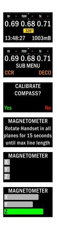
Press and hold the right button and switch the compass on. With the compass activated, press the left and right buttons simultaneously to show the menu options.
