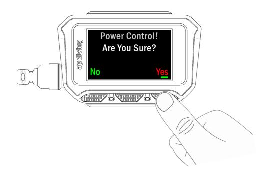
The Power Control allows the shutdown of either of the controllers or the whole system, except when underwater.
