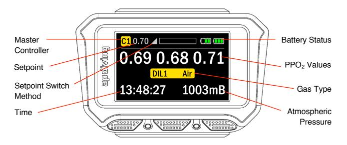
Following a successful calibration the 2020 Colour Display will enter 'Surface Mode'.
