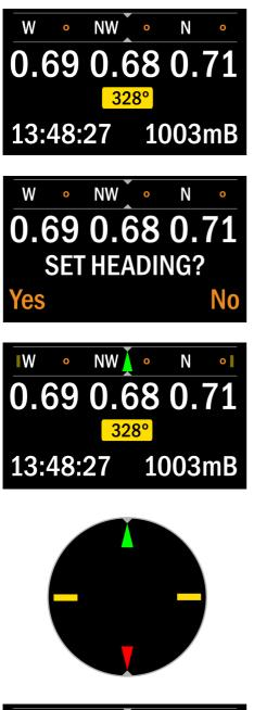
vs o sw o w o ∧ 0.69 0.68 0.71 236° 13:48:27 1003mB Once the compass is activated a heading can be set by holding the right button for 2 seconds
