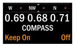
Once the Compass is activated either with or without a set heading, it can be turned off by again holding the right button for 2 seconds to display the 'Set Heading?' option.
