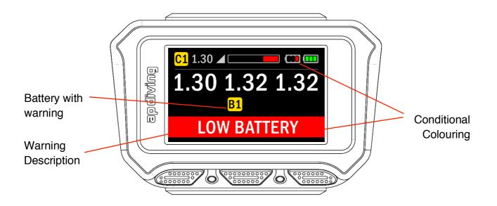
The 2020 Colour Display shows which Controllers (or Batteries) are generating the warning and the warning is displayed in high contrast white on red.
