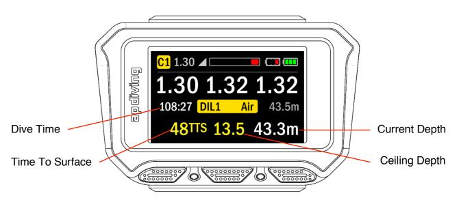
The time to surface and ceiling depth are shown in yellow, highlighting the decompression obligation currently in place. The scrubber monitor and B1 battery status in this example are in red showing a low battery issue and poor condition of the  $CO_2$  scrubber.
