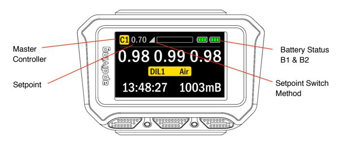
The Setpoint Switch Mode icons are shown below: manual, automatic, gradual and forced low (respectively). If the diver selects to switch to Open Circuit, the 'OC' symbol will replace the Setpoint mode icon.
