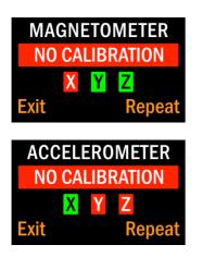
If the handset is not rotated sufficiently enough during either calibration process to give an accurate calibration, a 'No Calibration' screen will be displayed. This will indicate which plane did not receive enough rotations with a red box. In the first example the X plane caused the failed calibration and in the second example, it was the Y and Z. Simply select 'Repeat' and attempt to rotate the handset again or select 'Exit' to continue without calibrating the compass.
