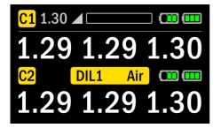
The top line controller 1 information, controller 2 information and diluent can be seen at any time whilst the compass is active by holding the left button for 2 seconds.
