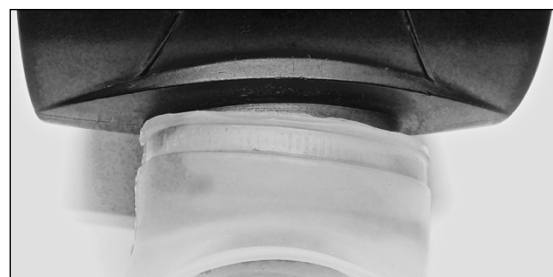
INCORRECT : no horizontal alignment
