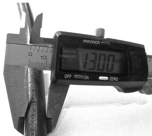
New standard type 13 mm diameter MP hose
