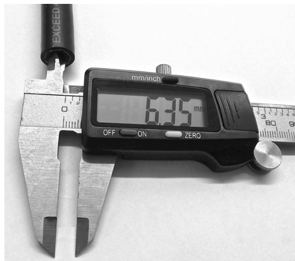
New standard type 6.35 mm (1/4") bore MP hose
