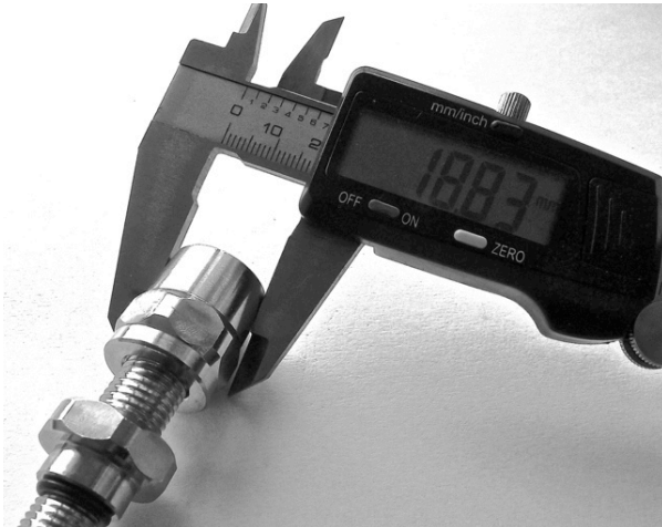
Old type hose end (AP150 hose): 18.8 mm diameter
