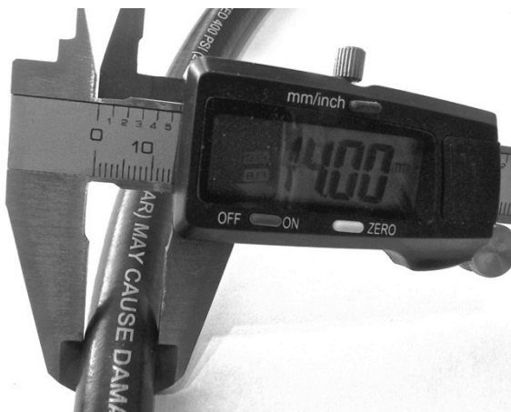
Old Auto Air-only 14 mm diameter MP hose
