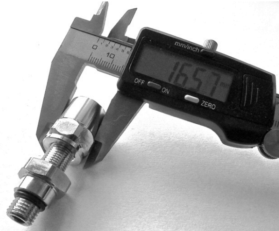
New type hose end (EV50 hose): 16.5 mm diameter
