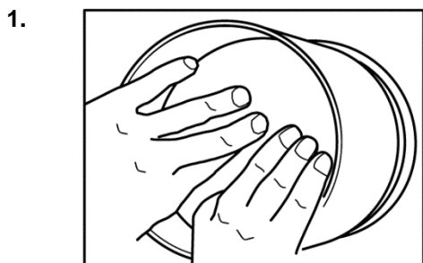
Ensure the filter scrim is clean and undamaged. Push in into the cartridge as far as it will go.
